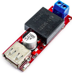
Fig. 11. KIS-3R33S 5V solar panel regulator[18]
