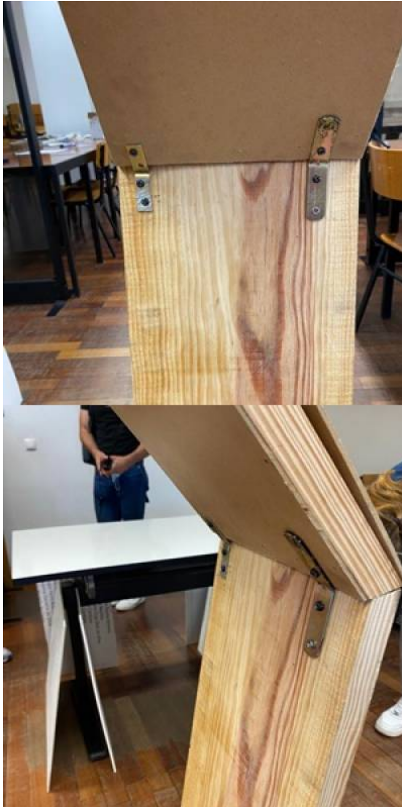
Figure 57: Internal connection between pillar and upper part of prototype
