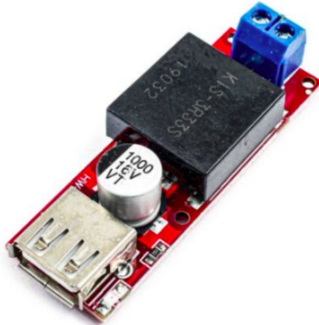
Figure 47: KIS-3R33S 5V solar panel regulator.
